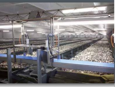
"Picking bridges" in combination with the central conveyor system will transport the full trays to the processing area.
