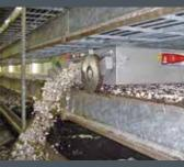
Stem removing machine VR.020
