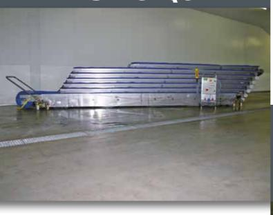
Inclined conveyor combined with a central conveyor to transport mushroom from the growing rooms to the processing area.
